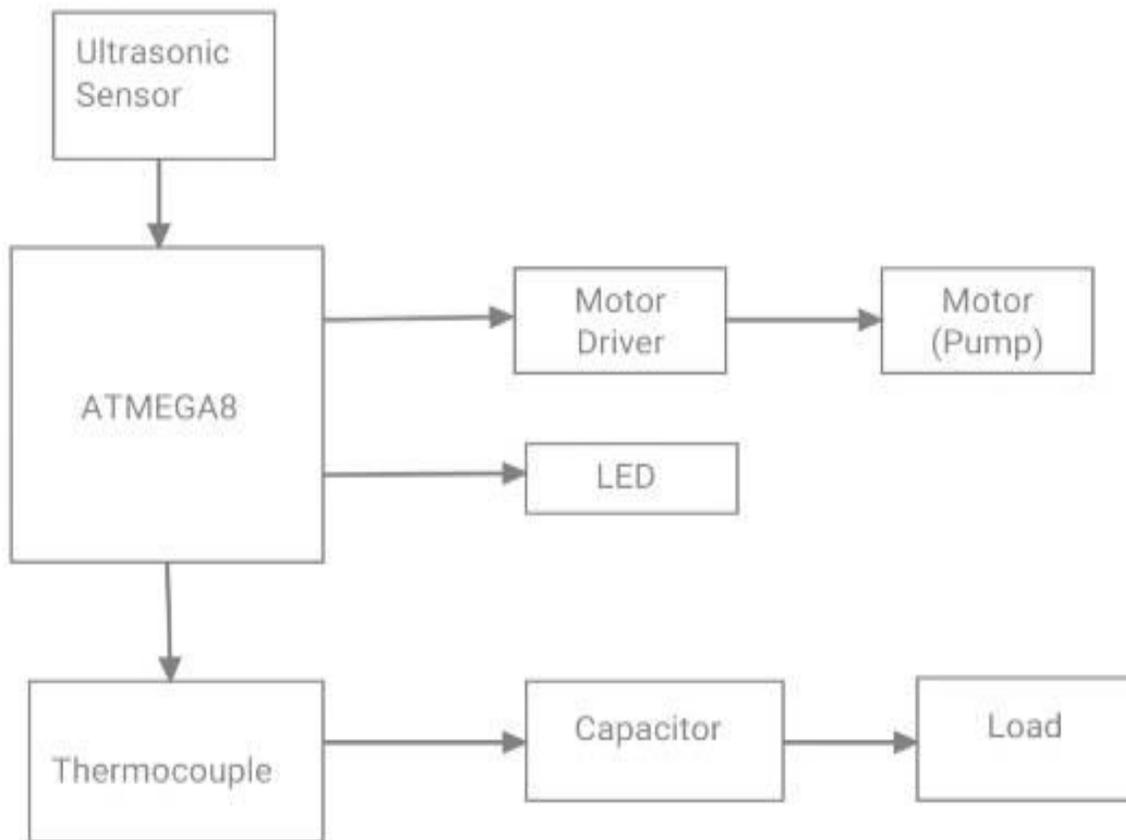
Fig: 1 Block Diagram of the system.
